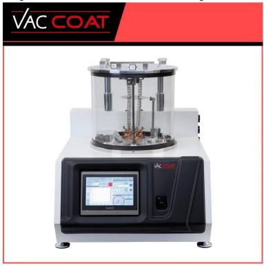
The DTT is a desk top, turbo molecular-pumped thermal evaporator for vacuum deposition of thin films. The triple-source evaporation with evaporation source (boat / basket / coil) selection system is ideal for deposition of multilayer or alloys.
